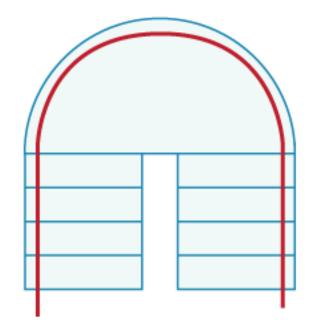
A U-shaped stair lift will incorporate two straight rail pieces connected by at least two curved rail pieces. The amount of straight and curved rail pieces is completely dependent on the size of your staircase, if there are landings, and which side the chair will be on. Rail pieces are seamlessly joined together by spiral pins after the leg bases are mounted to the stairs. Leg bases provide the height and stability needed to keep your stair lift safe.
