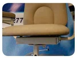
**IMPORTANT:** Be aware that the GEAR RACK of the CHASSIS RAIL is not yet timed with the GEAR RACK of the LOWER RAIL ASSEMBLY. THE UNIT WILL 'FREE WHEEL' TO THE LOWER ASSEMBLY WHEN IT IS DRIVEN OFF THE TOP GEAR RACK.
